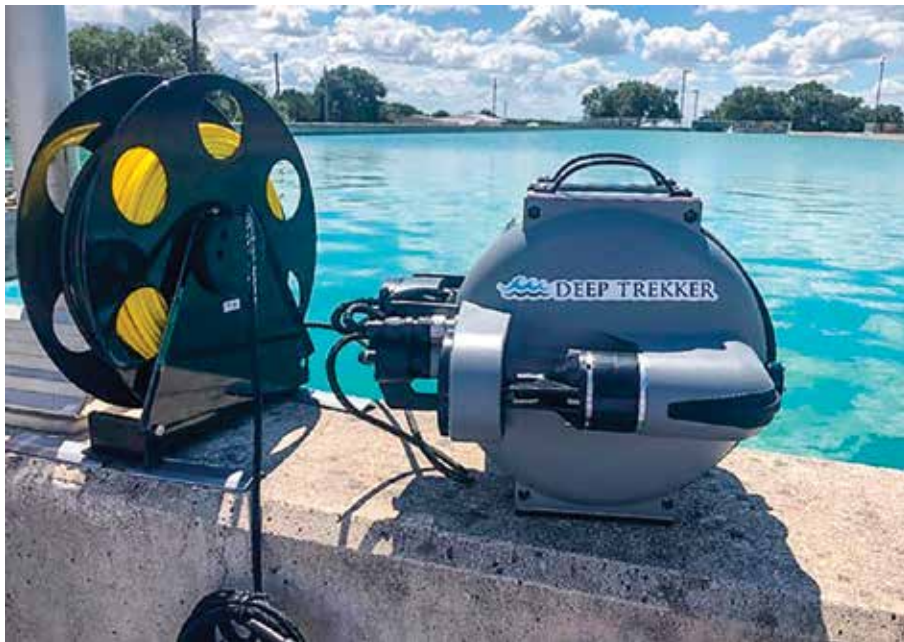
Figure 4 – Deep Trekker Robotic CCTV at Western Canyon WTP.
