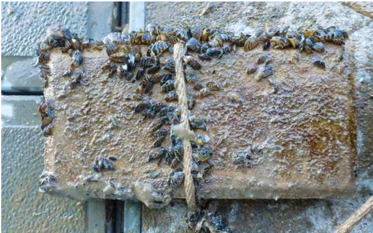
Figure 1 - Colonized McMahan Style Zebra Mussel Sampler at Canyon Lake.
