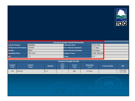
Here you can see the pH, disinfectant residual, sampler name, and temperature. This information will always be present on chemical results.
