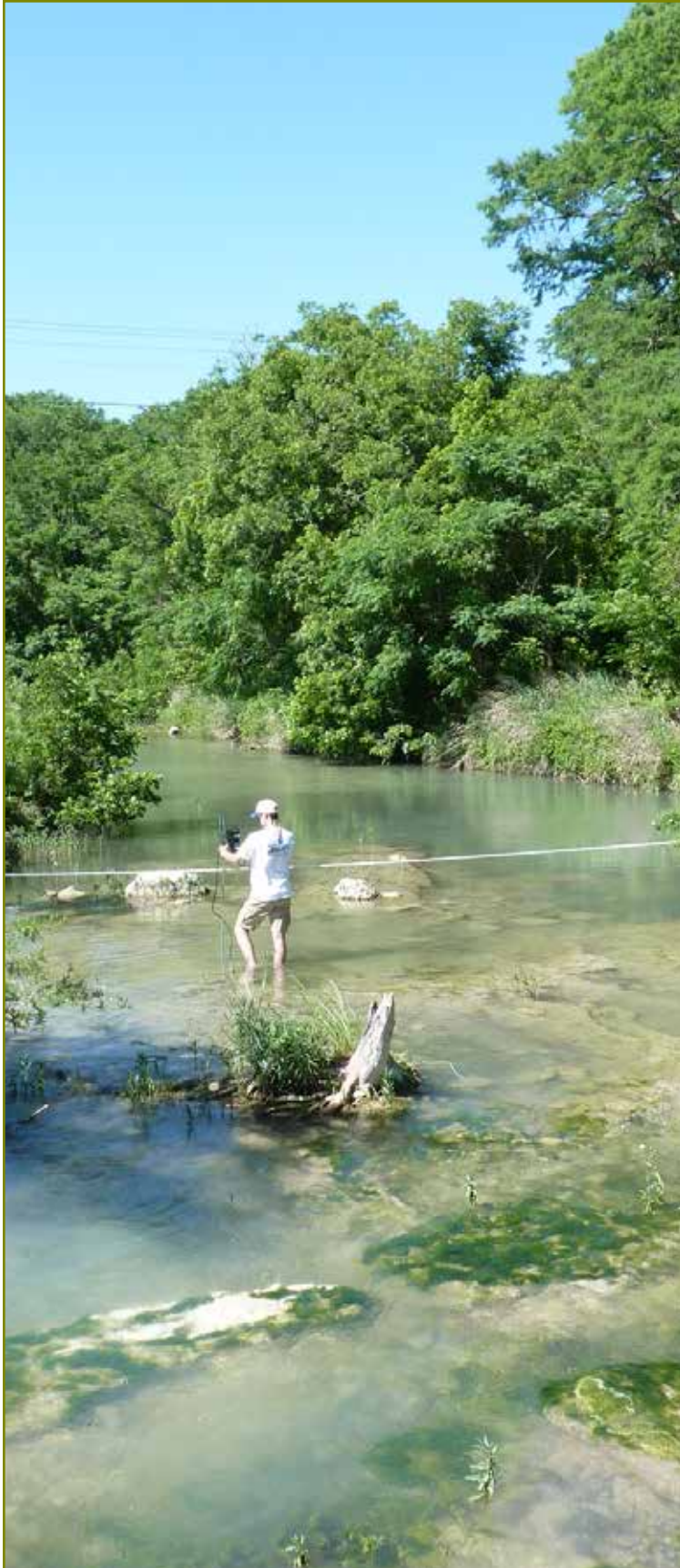
Travis Linscomb with UGRA measuring flow in Johnson Creek Photo by Tara Bushnoe
